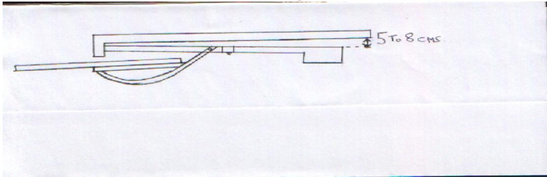
**Under no circumstances should the motor head be above the front mounting bracket.**
